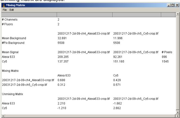
h) Save the data to disk by using the "File->Save As..." command in the File menu of the Mixing Matrix window.
