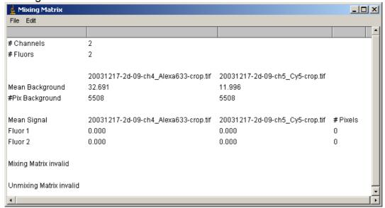
d) To measure the relative contributions of fluorochrome 1 (here Alexa 633) to the fluorescence channels, first click onto the right arrow of the lower control in the plugin window. The text next to it changes from "Background" to Fluor 1. You can give the fluorochrome a more intuitive name in the adjacent text box. Then draw a ROI around the respective reference object.
