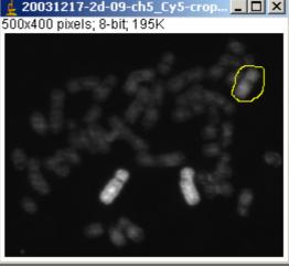
The ROI mostly contains pixels of the reference object, but also background pixels or pixels of other objects. To segment the reference object, adjust the threshold slider in the plugin window for a channel, where the object is best visible
