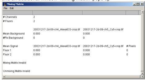
c) To measure the background in all images, select a ROI, which has only background signal in all images. It is sufficient to do this in one image. The ROI is drawn synchronously in all images. Then double-click into the ROI.
