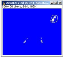
e) To perform the actual measurement, double-click into the ROI in the image, where you segmented the reference object. The plugin measures the mean intensities of the pixels within the ROI, which are above the threshold in this image and the mean intensities of the same pixels in all other color channels.
